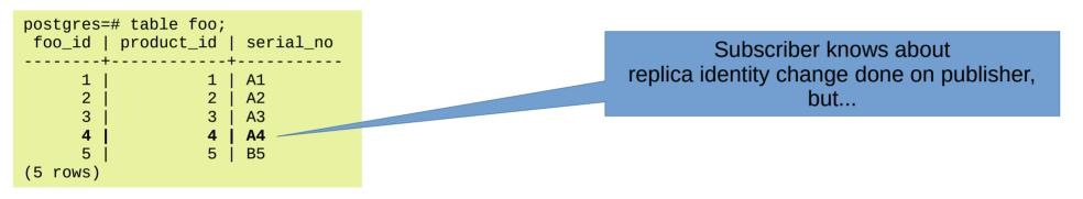
LOG: logical replication apply worker for subscription "sub\_test" has started ERROR: **publisher did not send replica identity column expected** by the logical replication target relation "public.foo" LOG: background worker "logical replication worker" (PID 6526) exited with exit code 1
