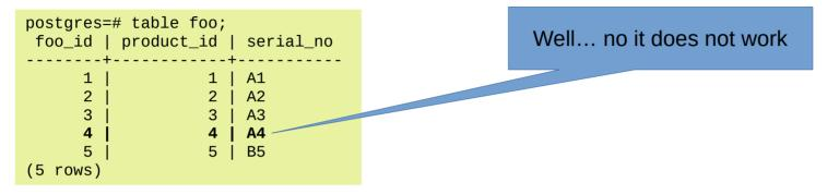
LOG: logical replication apply worker for subscription "sub\_test" has started ERROR: **publisher did not send replica identity column expected** by the logical replication target relation "public.foo" LOG: background worker "logical replication worker" (PID 6037) exited with exit code 1
